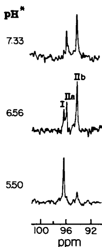
FIG. 5. 13 C-NMR spectra at 50.3 MHz of the nicotinamide carboxamide carbon in the dihydrofolate reductase–folate–NADP + complex at various pH values, showing the three coexisting states I, IIA, and IIB. From reference 310.
